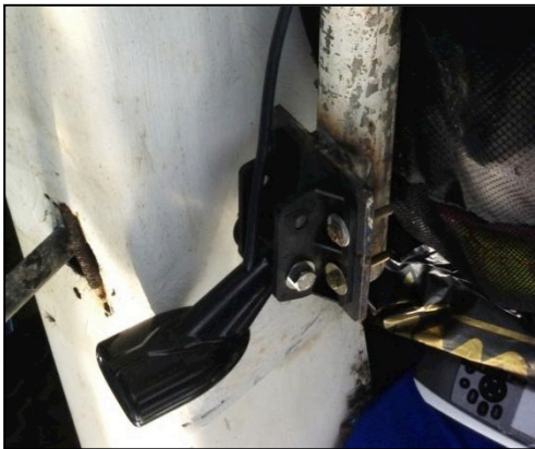
Figure 2.14 Lowrance transducer on a side-mount
