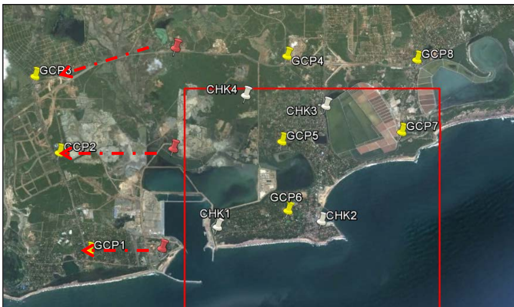
Figure 3.13 GCPs relocated in the field
