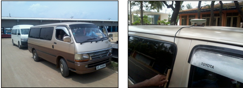
Figure 3.9 GPS receiver attached to the van, its height from antenna to the ground was measured using a measuring tape
