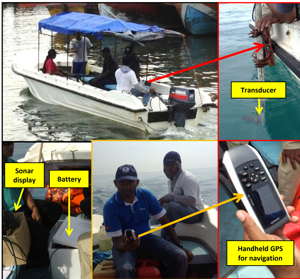
Figure 2.13 Sonar setup on NARA skiff
