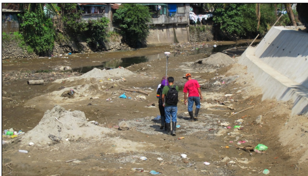
Figure 5.2 RTK GPS survey along a dried up river
