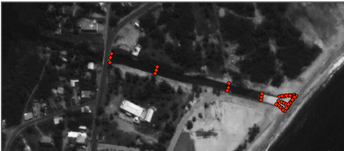
Figure 5.3 RTK GPS survey along the canal on 4 April 2013
