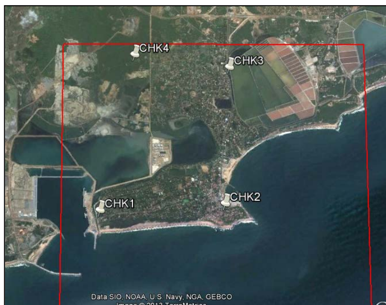
Figure 3.5 Checkpoints for aerial photogrammetry
