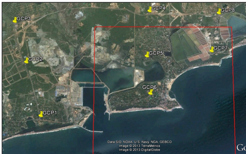
Figure 3.4 GCPs for aerial photogrammetry
