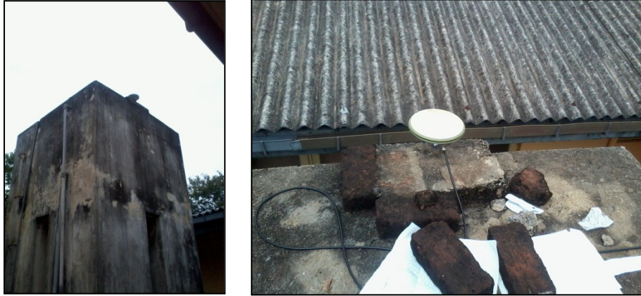
Figure 3.8 RTK GPS base station set up at benchmark number A025 and broadcasting correction data through radio
