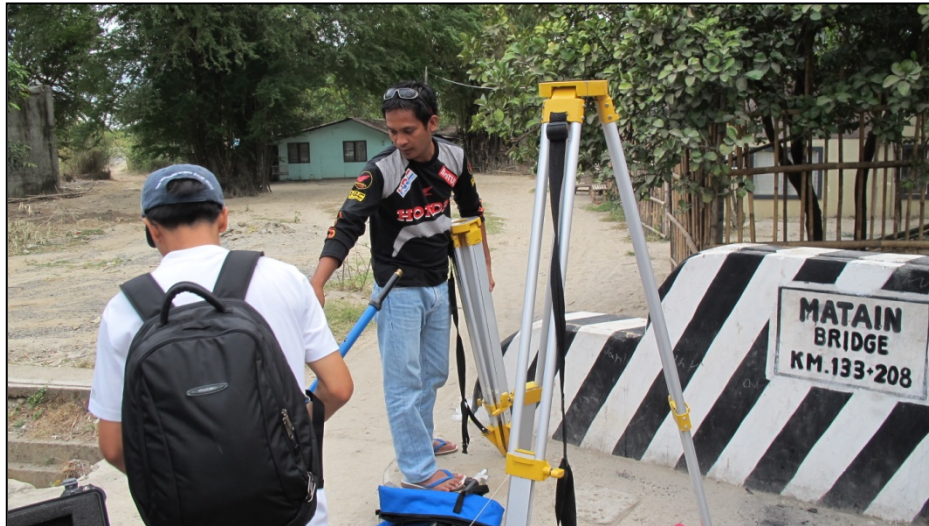
Figure 3.16 Base station set up on the elevation benchmark on the morning of 22 January 2013
