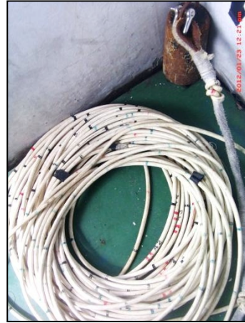
Figure 2.28 Calibrated rope to check sounding data
