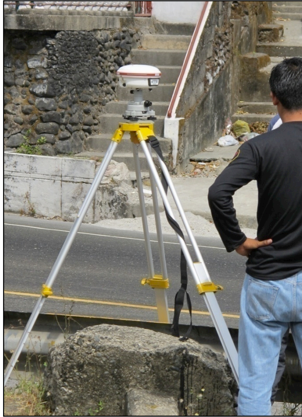
Figure 3.4 GPS setup on a known horizontal benchmark (ZBS-3197)
