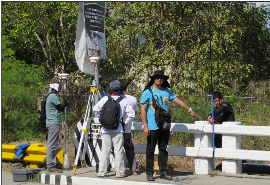
Figure 4.1 Base station set up at CHK1
