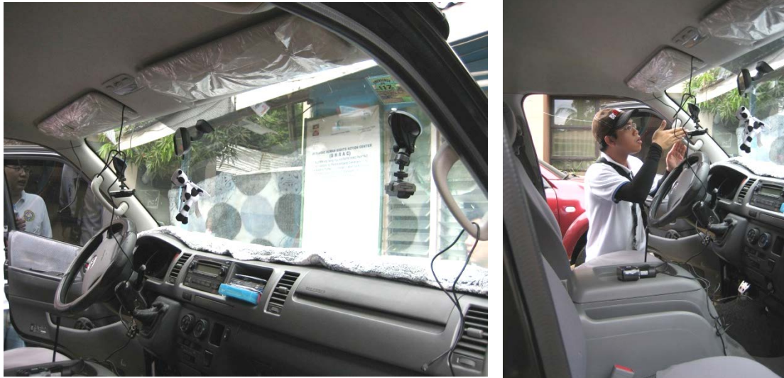
Figure 6.15 VDO camera with GPS receiver mounted on the survey vehicle
