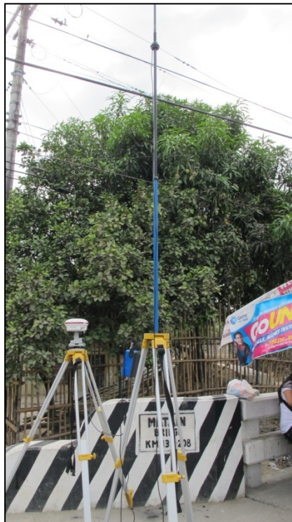
Figure 3.8 RTK GPS base station set up at GCP5 and broadcasting correction data through radio
