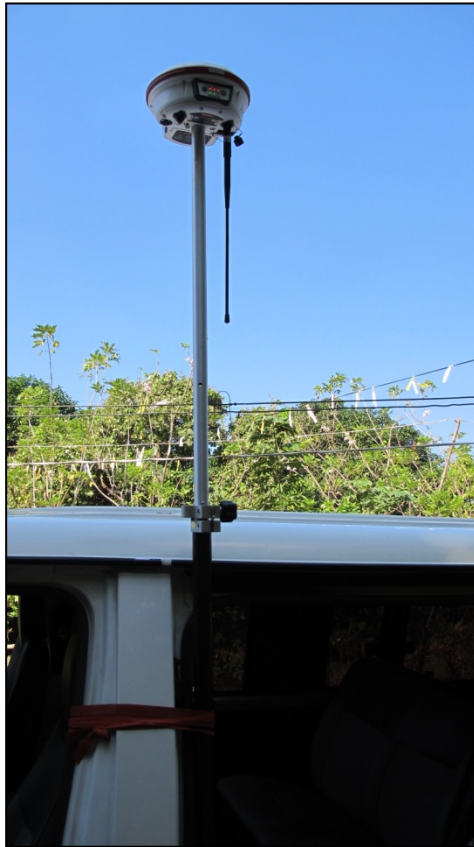
Figure 3.9 GPS receiver attached to the van; height from antenna to ground was measured using a measuring tape
