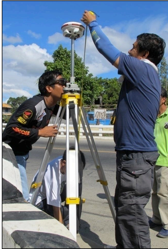
Figure 3.2 GPS setup on a known elevation benchmark (BM ZA-17A)
